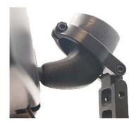
4 - Reattach the right side of the mount. Make sure the small lock washer is still on the lower screw and tighten untill the screw is fairly snug. Leave the top screw loose so the mount can slide towards the windshield around the large diameter of the mirror stem.
